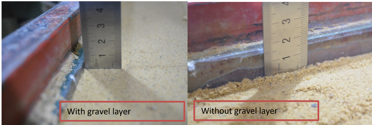
Plate 4: The differences in subsidence between cases using gravel and without a tiny gravel protective layer
